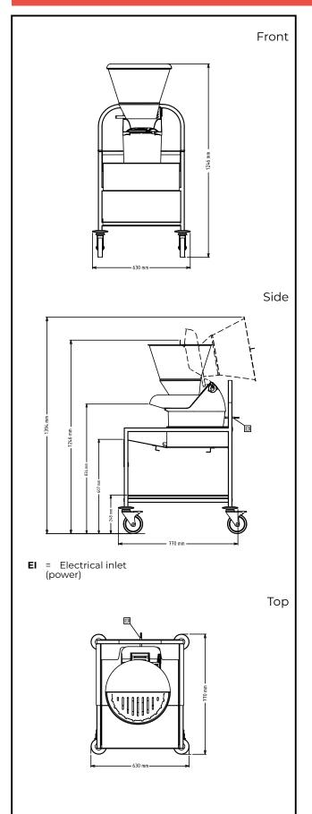
Electric Supply voltage: 200-240 V/1N ph/50/60 Hz Electrical power, max: 0.5 kW **Total Watts:** 0.5 kW Capacity: Performance (up to): Key Information: External dimensions, Width: 630 mm External dimensions, 770 mm Depth: External dimensions, Height: 1250 mm
